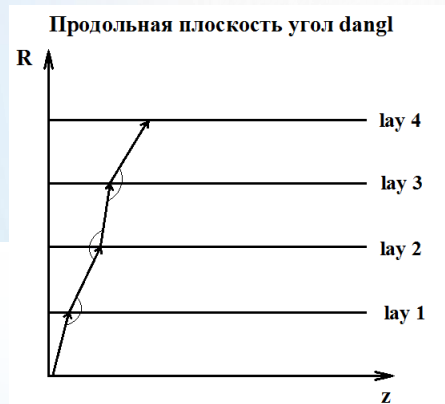
Fig. 11. Schematic representation of the angle d\text{angl} in the longitudinal plane
