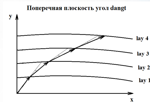
Fig. 12. Schematic representation of the angle d\text{angt} in the transverse plane
