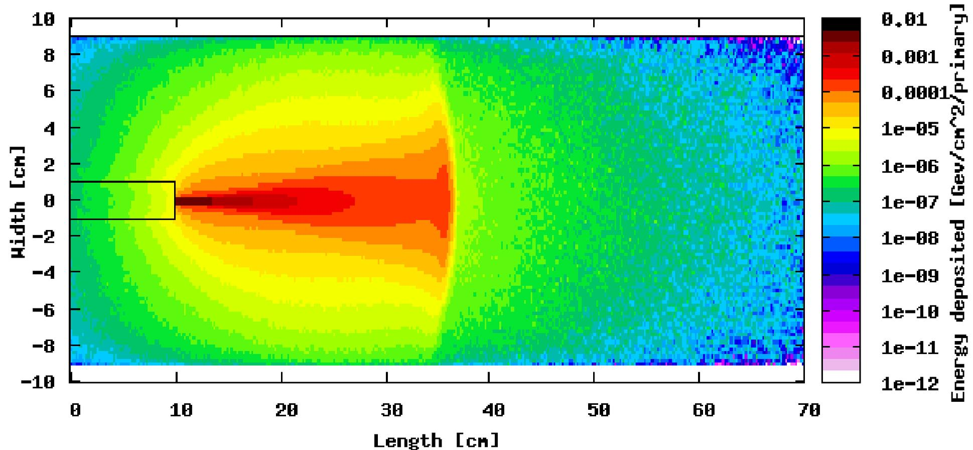
Energy deposition in a cylindrical lead target of 70 cm long and 9 cm in radius target irradiated by 600 MeV electrons
