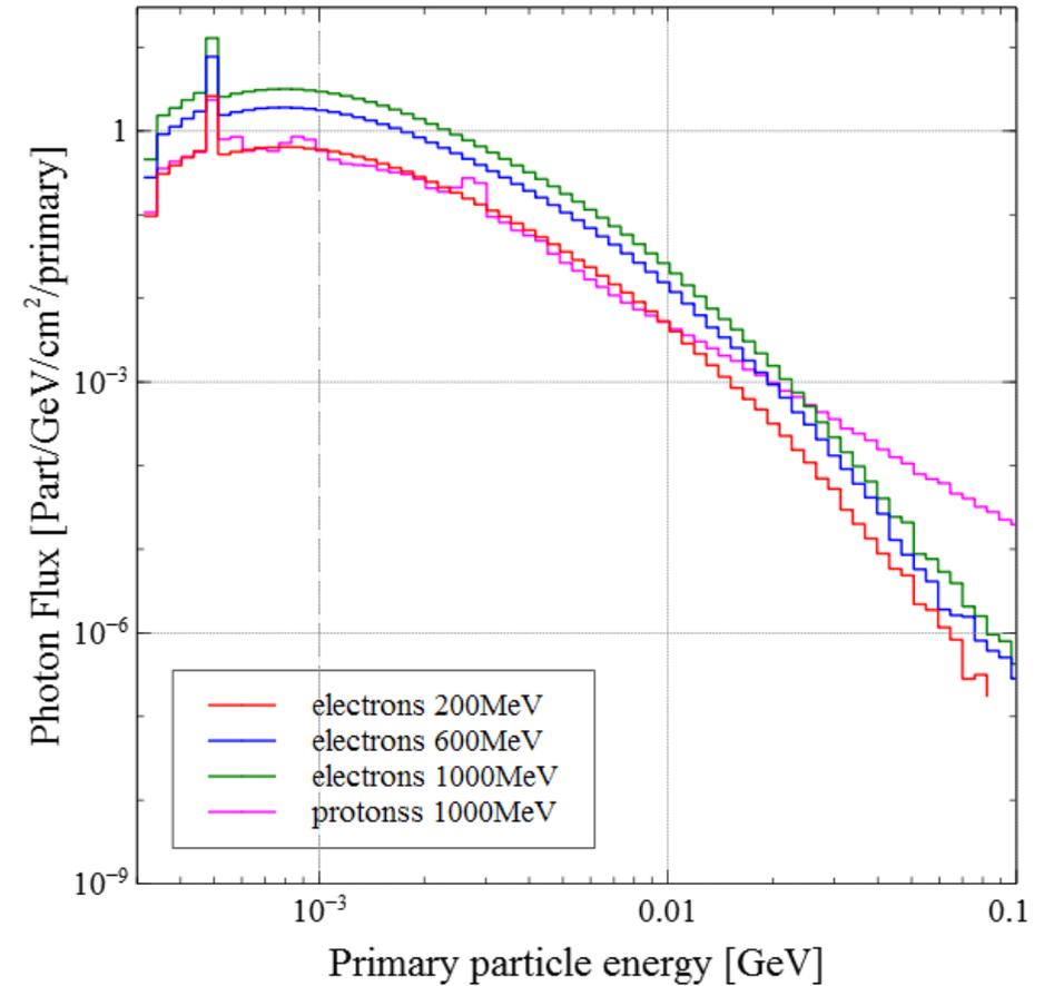
Energy spectra of neutrons (left) and photons (right) produced by electrons of energy 200, 600 and 1000 MeV and protons at 1000 MeV in a cylindrical lead target of 70 cm long and 9 cm in radius and escaping from it. Calculated by means of FLUKA.
