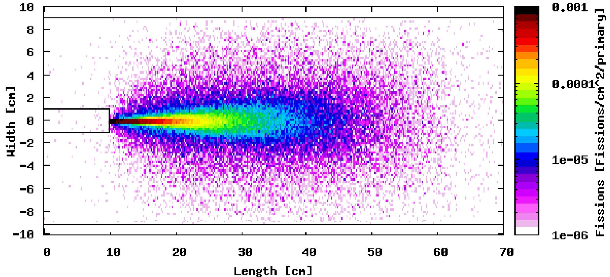
Energy deposition in a cylindrical lead target of 70 cm long and 9 cm in radius target irradiated by 1 GeV protons
