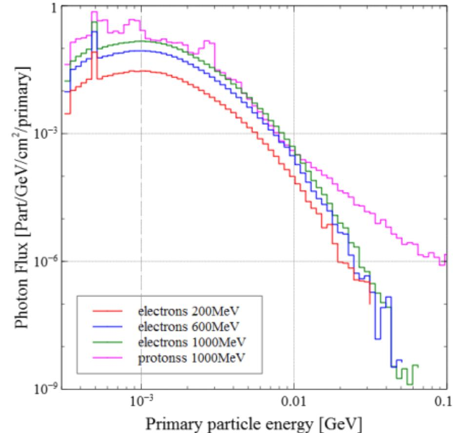
Energy spectra of neutrons (left) and photons (right) produced by electrons of energy 200, 600 and 1000 MeV and protons at 1000 MeV in a cylindrical tungsten target of 70 cm long and 9 cm in radius and escaping from it. Calculated by means of FLUKA.
