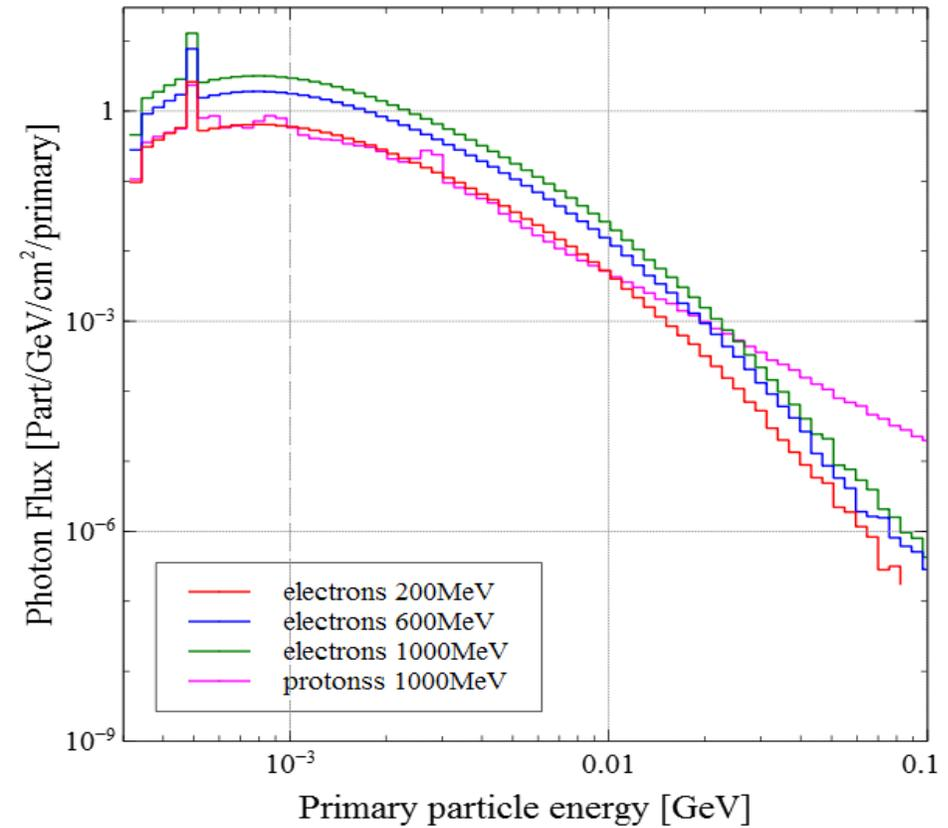
Intensity of neutrons (left) and photons (right) created in a cylindrical lead target of 3.34 cm long and 3.34 cm in radius by electrons of energy from 30 MeV to 1000 MeV (calculated by using MCNPX)
