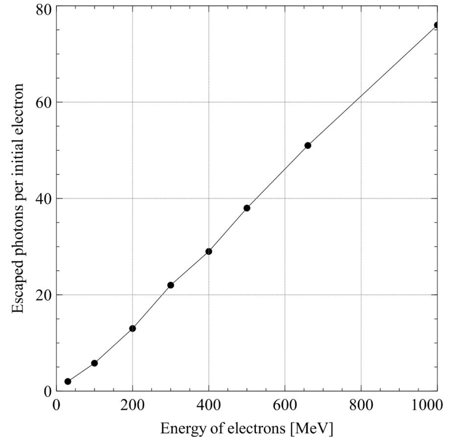
Yields of neutrons (left) and photons (right) created inside the cylindrical lead target of 70 cm long and 9 cm in radius by electrons of energy from 30 MeV to 1000 MeV calculated by using MCNPX.
