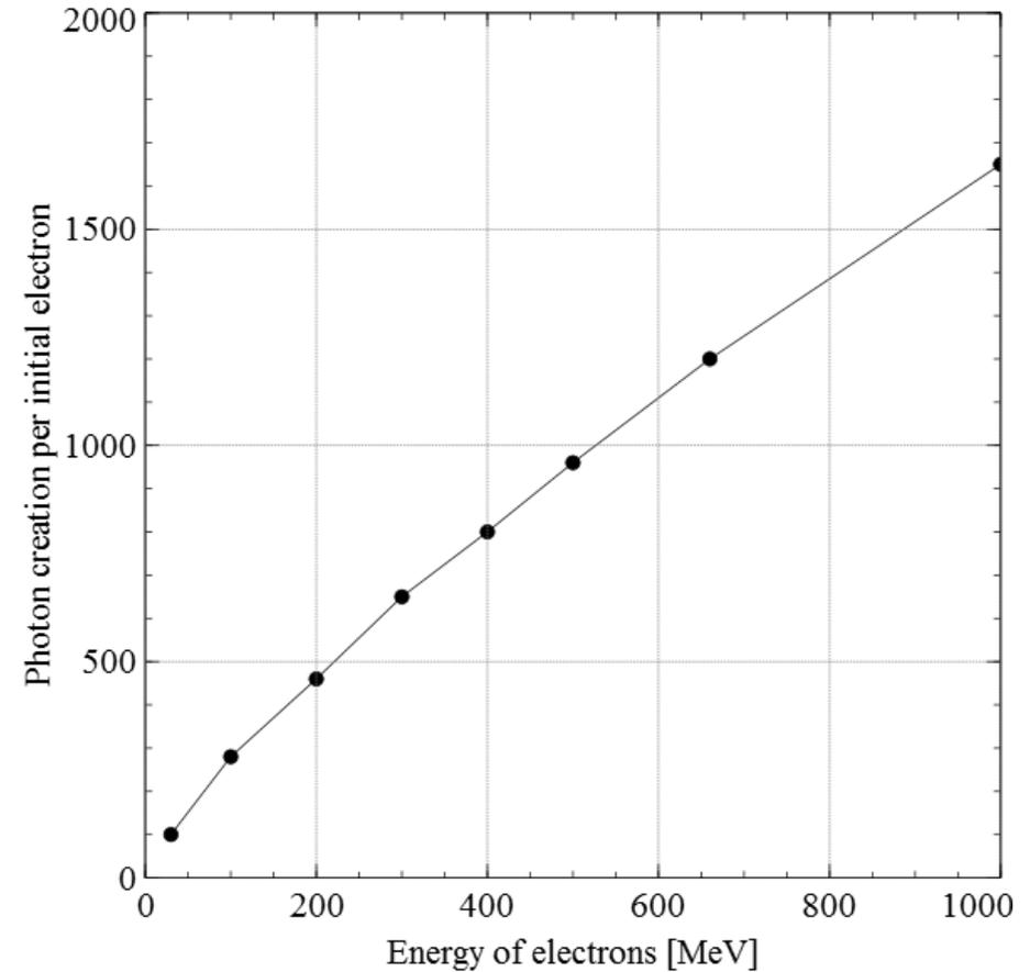
Intensity of neutrons (left) and photons (right) escaping from a cylindrical lead target of 3.34 cm long and 3.34 cm in radius by electrons of energy from 30 MeV to 1000 MeV (calculated by using MCNPX)
