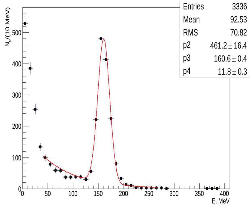
**Energy spectrum of particles, registered by a single BGO element of SPEC. The peak in the region  $\sim 160$  MeV corresponds to MIP particles**
