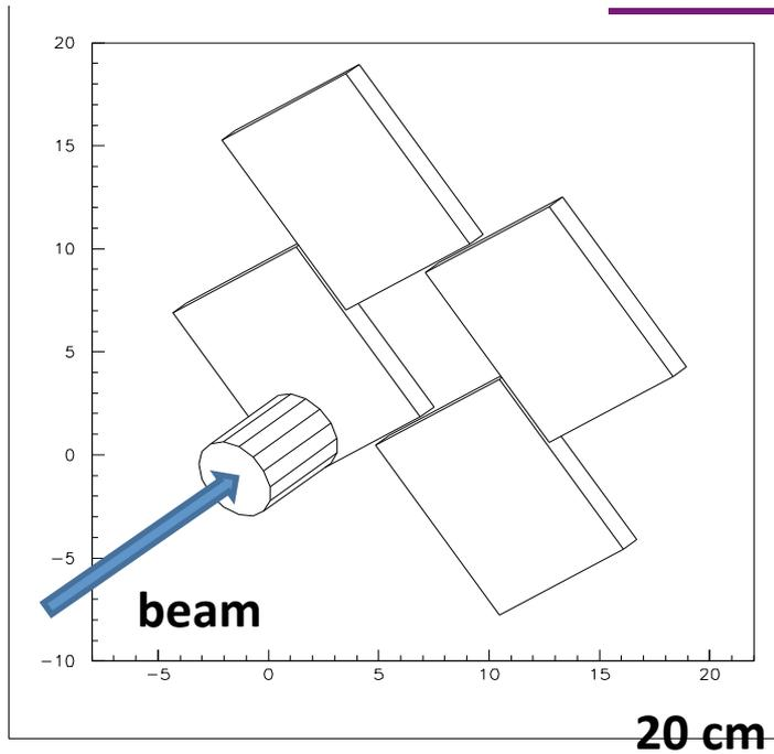
**Target  $^{12}\text{C}$  and trigger hodoscope of multiplicity**
