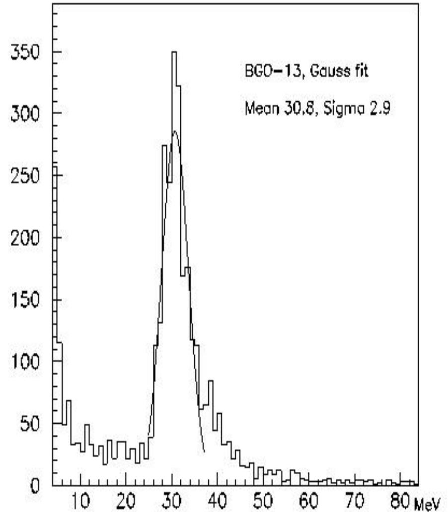
run116, E-loss of cosmic muon in 30mm BGO(13),  $dN/dE$ ,  $dE=1\text{MeV}/\text{ch}$ .
