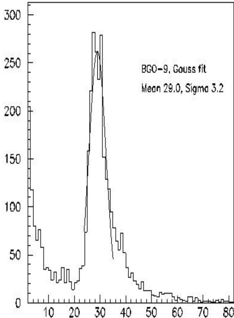
run116, E-loss of cosmic muon in 30mm BGO(9),  $dN/dE$ ,  $dE=1\text{MeV}/\text{ch}$
