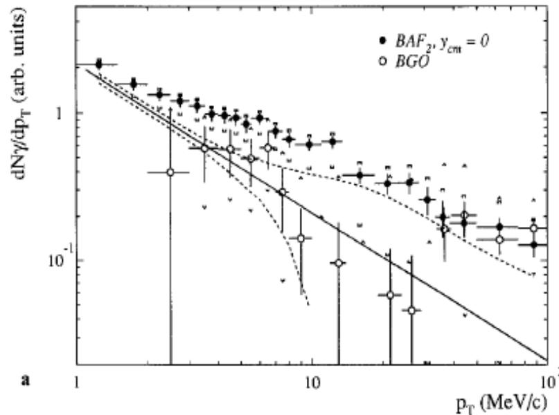
SP yield has been measured at WA91 setup in  $\pi p$ ,  $pp$ , 280 ÷ 450 GeV/c to test results of OMEGA setup . It was “clear” experiment, it was selected events:  $N_{ch} \leq 8$ . Photons registered by conversion pairs in lead layer.
