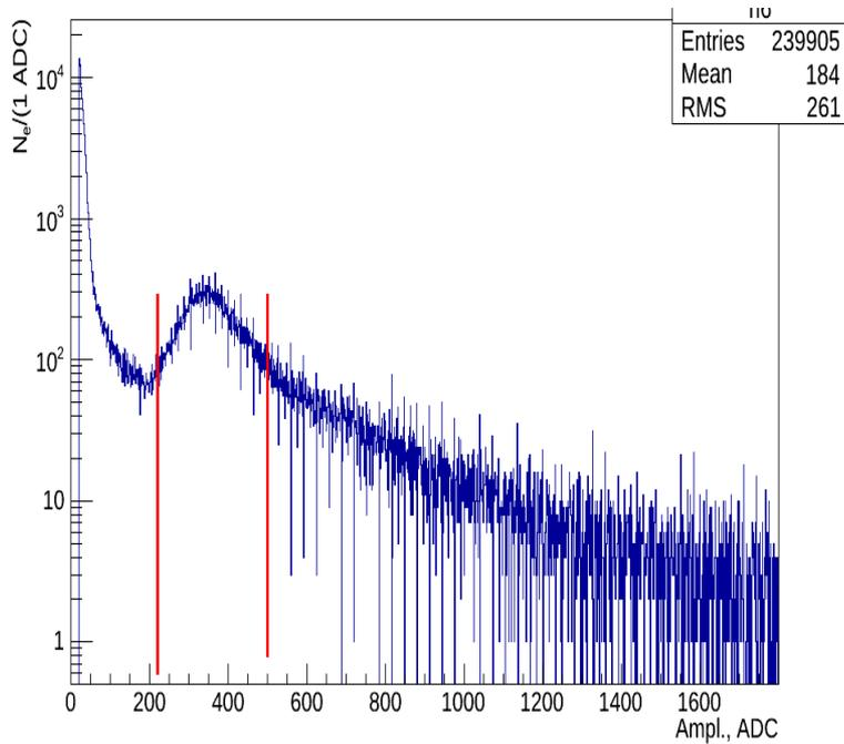
**Amplitude spectrum of signals from front veto-detector of SPEC**
