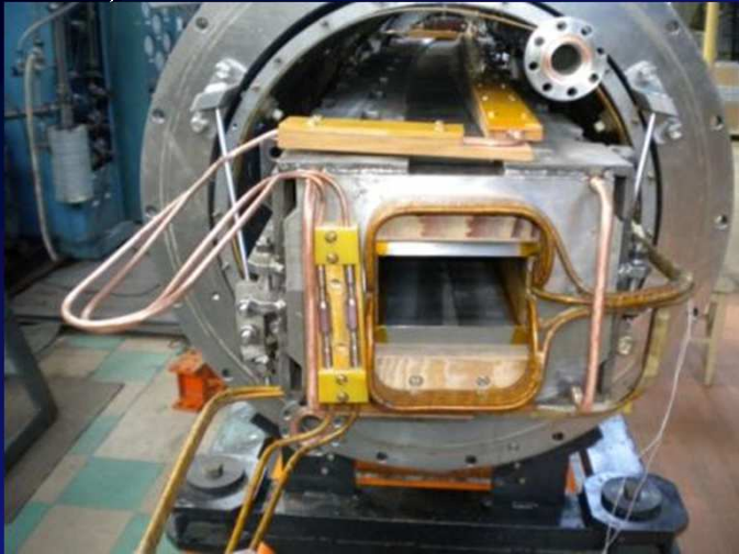
Booster dipole at cryo-test (9690A) and magnetic measurements
