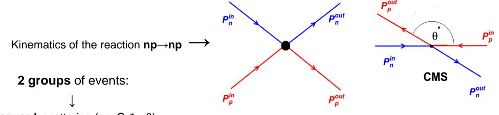
**Forward** scattering  $(cos\Theta_p^* < 0)$ reaction without charge exchange ("0.ex"), variable  $t=(P_p^{in}-P_p^{out})^2$
