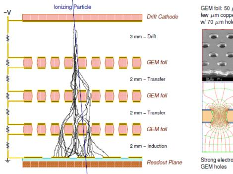
GEM foil: 50  $\mu$ m Kapton + few  $\mu$ m copper on both sides w/ 70  $\mu$ m holes, 140  $\mu$ m pitch
