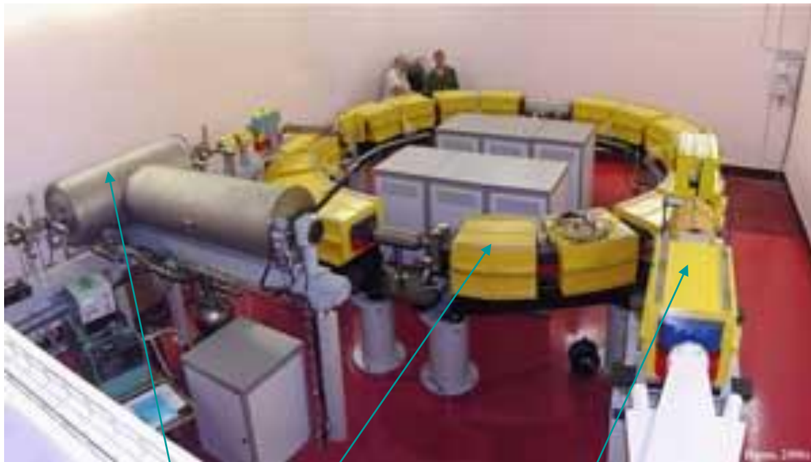
1. Injector; magnet; 2. Accelerator ring. 3. Scanning magnet;
