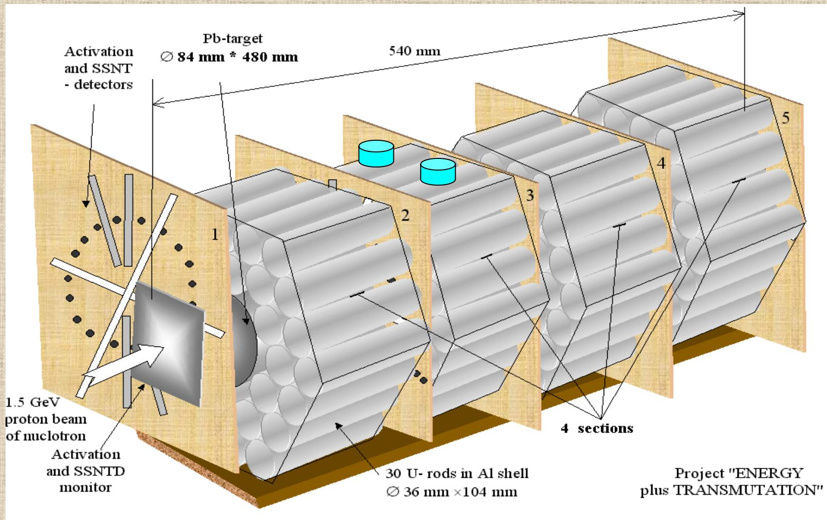
Photography of “Energy&Transmutation” Pb/U assembly outside the shielding before fixing of detectors
