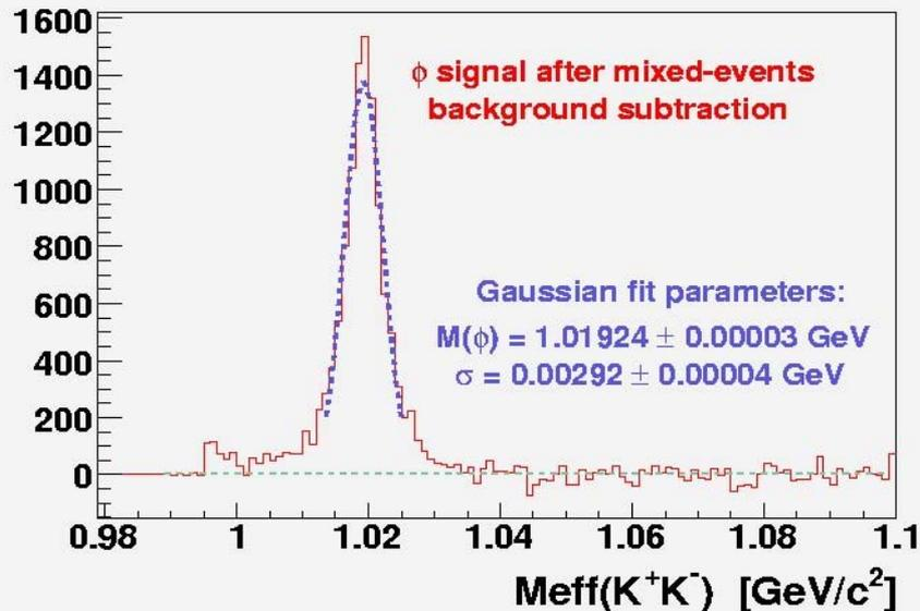
$7.3 \times 10^6$  events were analyzed with the ITS, TPC and TOF for the tracking and kaon identification.
