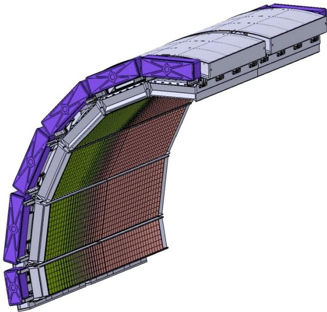
Lead scintillator sampling calorimeter
