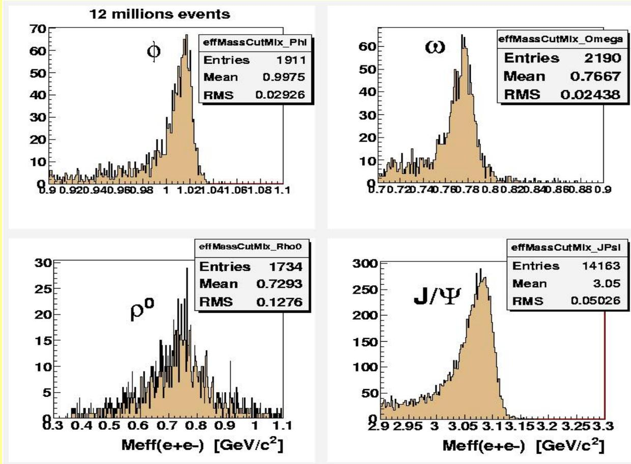
Effective mass ( $\text{GeV}/c^2$ ) distributions of ( $e^+e^-$ ) pairs from decays of  $\phi$ ,  $\omega$ ,  $\rho^0$ ,  $J/\psi$ .
