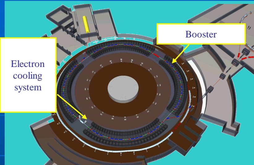
Design and parameters of booster, including wide accessible energy range, possibility of the electron cooling, allow to form dense and sharp ion beams. System of slow extraction provides slow, prolonged in time ion extraction to the target with space scanning of ions on the target surface and guaranty **high controllability** of experimental conditions.
