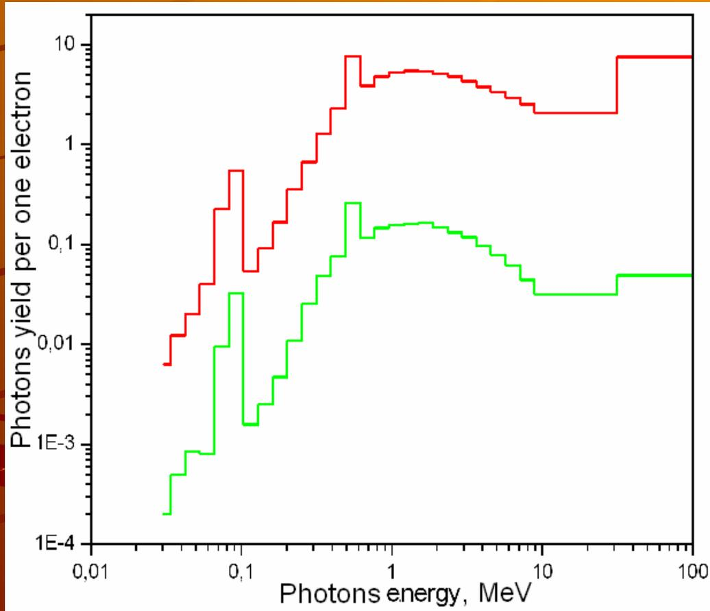
*Spectrum of photons produced by a single electron of energy 30 MeV (green) and 1000 MeV (red) in the lead target 3.34 cm along and 3.34 cm in diameter.*
