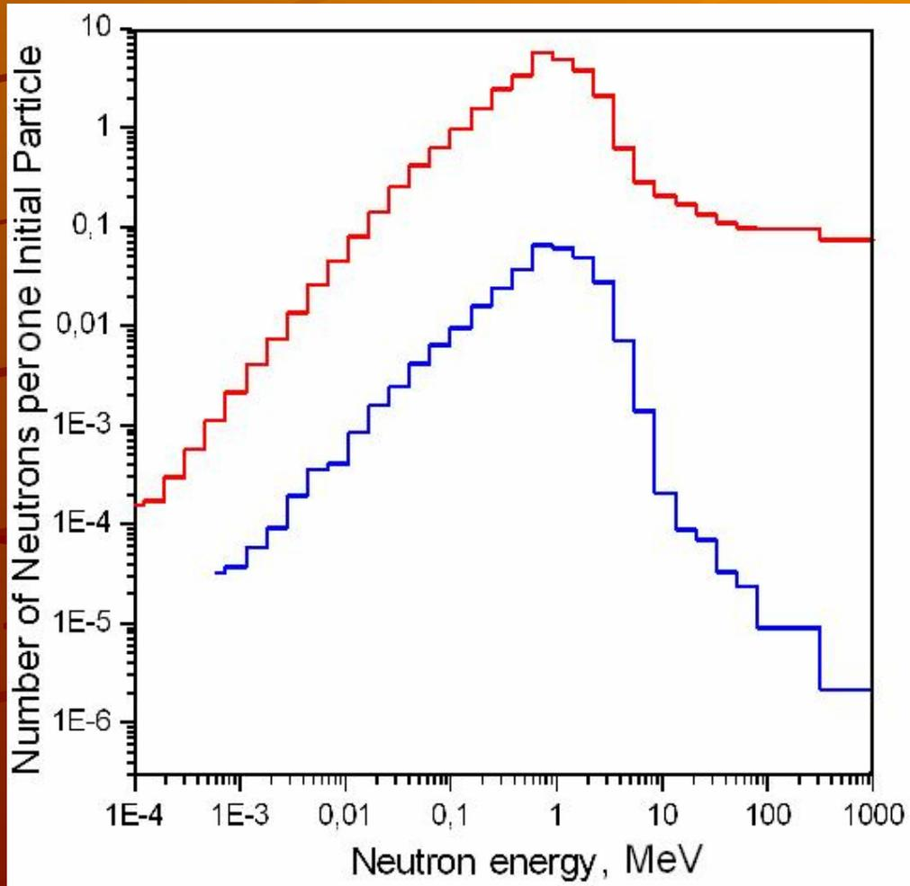
*Spectra of neutrons produced by single electrons (blue) and protons (red) of energy 1000 MeV in the lead target 60 cm along and 60 cm in diameter.*
