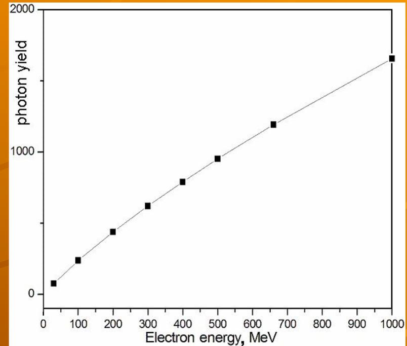
*Average multiplicity distribution of neutrons (left) and photons (right) produced by single electrons of energy from 30 to 1000 MeV in the lead target 3.34 cm along and 3.34 cm in diameter.*
