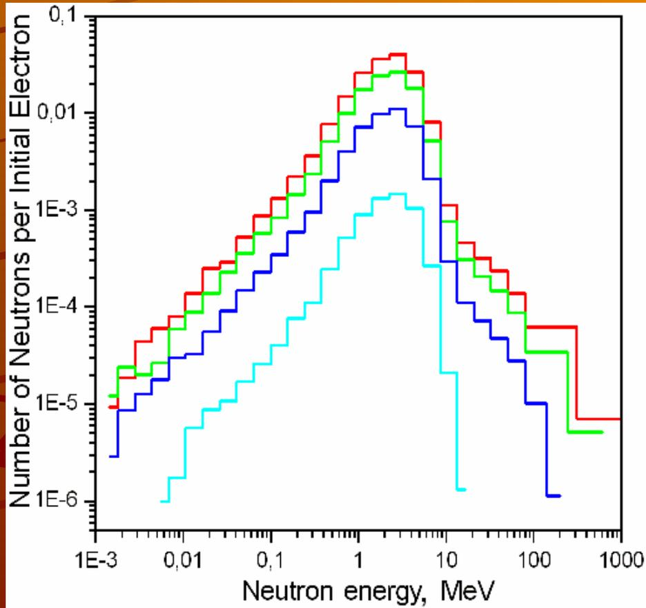
*Spectrum of neutrons produced by a single electron of energy 30, 200, 600, 1000 MeV in the lead target 3.34 cm along and 3.34 cm in diameter.*
