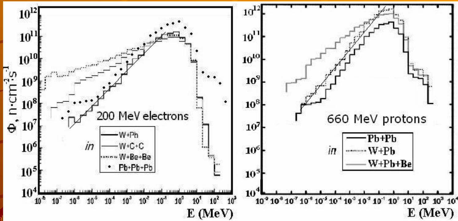
Energy spectra of neutrons produced in W and Pb central target rods of the assembly by 200 MeV electrons (left) and 660 MeV protons (right). Straight lines illustrate the fitting function  $(\Delta\Phi/\Delta E) \sim E^{0.81\pm 0.01}$ .
