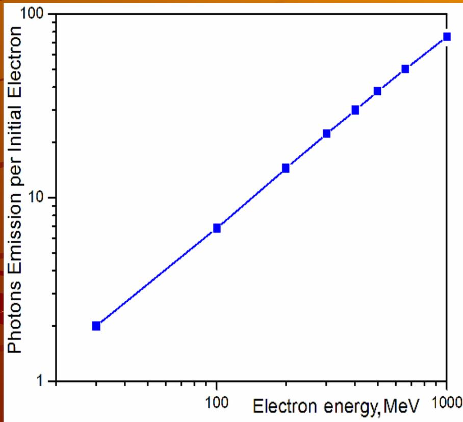
*Escaped photons produced by a single electron of energy from 30 MeV to 1000 MeV in the lead target 3.34 cm along and 3.34 cm in diameter.*
