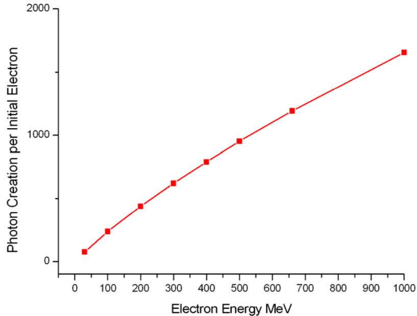
*Average multiplicity distribution of photons (produced by a single electron) of energy from 30 to 1000 MeV in the lead target 3.34 cm along and 3.34 cm in diameter.*
