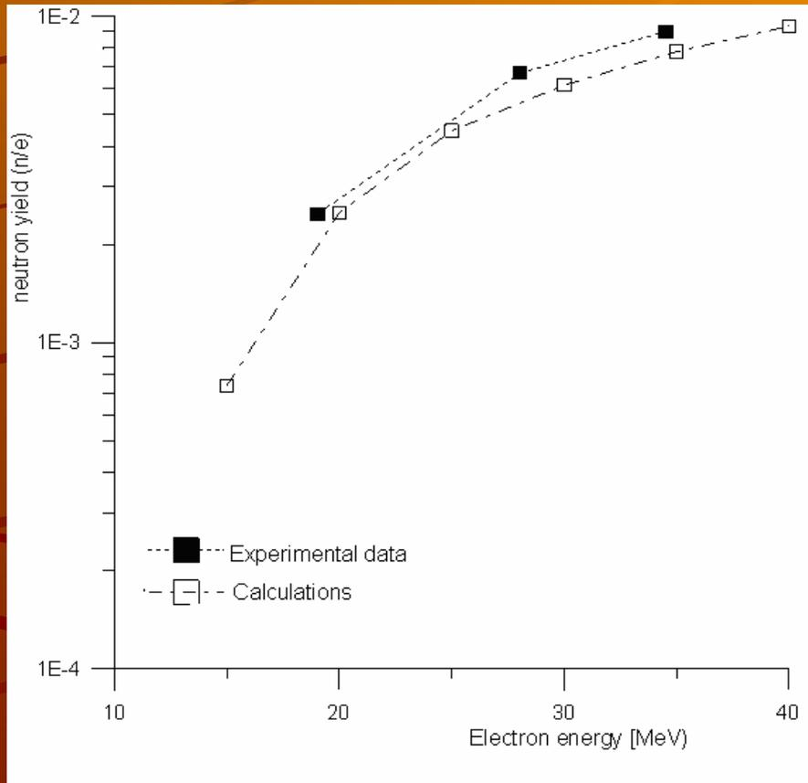
*Average multiplicity distribution of neutrons (produced by a single electron) of energy from 15 to 40 MeV in the lead target 3.34 cm along and 3.34 cm in diameter.*
