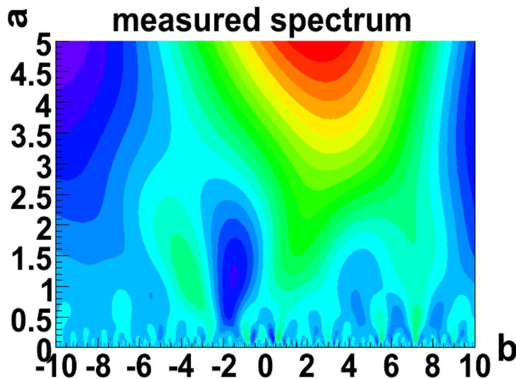
The MCHAT wavelet spectra of the previously shown event. Differences between the true and the corrected spectra seems larger on smaller scales which suggests they are primarily caused by statistical fluctuations.
