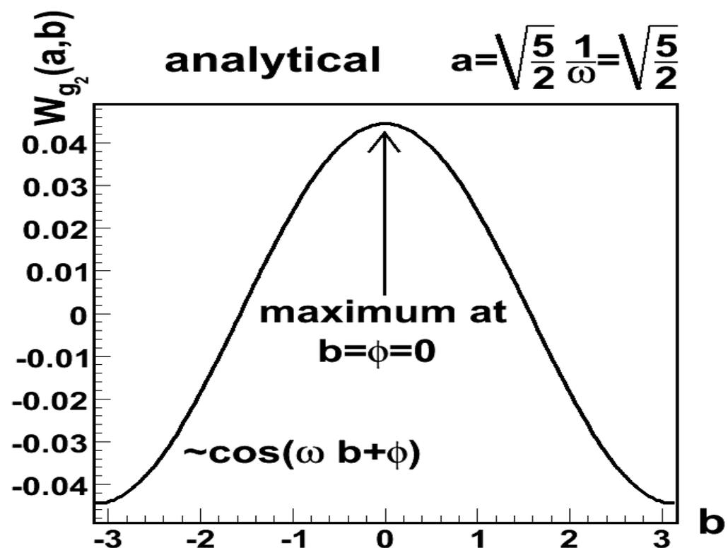
$b$  slices at the maxima of  $W_{\psi}(a,b)$  spectra for all the studied basis functions. The slices where the maxima are observed are done at the scales  $a$  which are displayed in the Figures. The plots are visual tests proving that the amplitude dependences on phase  $b$  have indeed expected cosine shapes.
