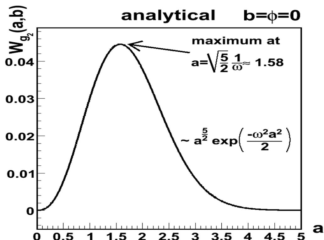
**a** slices at the maxima of  $W_{\psi}(a,b)$  spectra for all the studied basis functions. The plots indicate how is single Fourier frequency seen in scale space. Each  $\omega$  is represented by spectrum of scales  $a$ . Roughly  $\omega \leftrightarrow a_{max}$  (the position of maximum). The maxima for higher harmonics would appear closer to 0, since  $a_{max}(\omega) \propto 1/\omega$  for all the tested basis functions.
